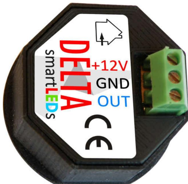
The sensor terminals are available on the terminal block at the back side of the device:
